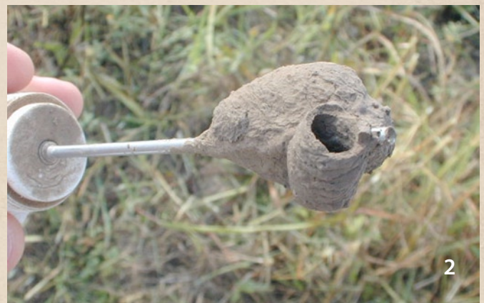
1. Mice damaged a sensor when they used part of a logger enclosure for a nest in fall 2007. 2. A mud dauber nest was found covering a temperature sensor in summer 2003. 3. Rodents, including gophers and prairie dogs, often damage sensors by digging them up or chewing on wires. This rodent hole was found in fall 2005.
